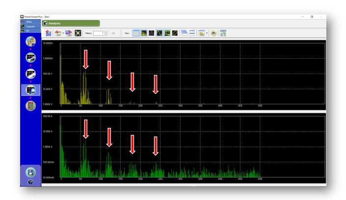
FIGURE 1: HARMONIC VOLTAGE PROFILE - FPWM – MV, NO CMF
